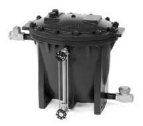
The Armstrong PT-200 Series Low Profile Pump Trap is a low maintenance, non-electric solution to move condensate or other liquids from low points, low pressures or vacuum spaces to an area of higher elevation or pressure. Condensate can be returned well above the 210°F (99°C) limit of conventional electric condensate pumps without the headaches of leaking seals or cavitation problems.
